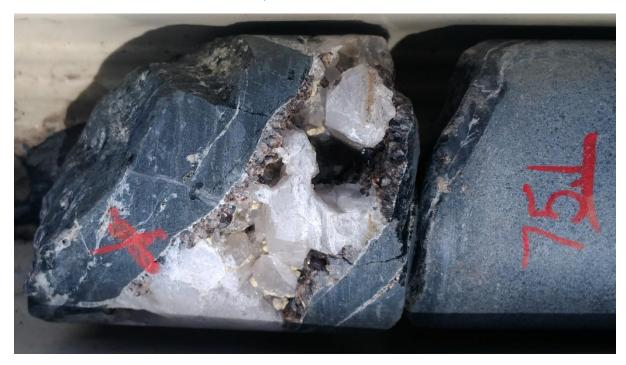
Photo: Quartz-Cassiterite vein at 75.1m in LDD003.
